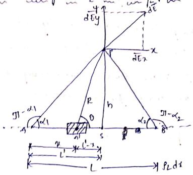
consider alength of wire AB of Lmi which has uniform charge continuously distributed through out the line. Its line charge density is Si. Let us determine electric field intensity with a line charge AB. from the figure the point p'is a distance of hmt. from S which is at a distance of it from end of A.
