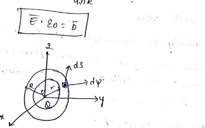
It state that, the surface integral of normal component of electric flux density (6) over any closed surface is equal to charge enclosed.
